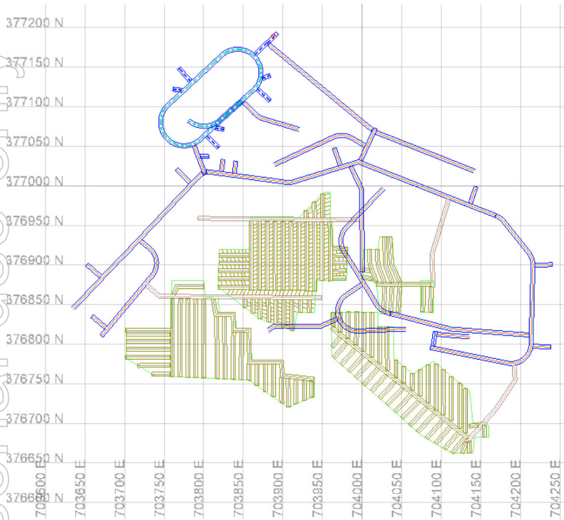
Figure 9: Typical flitch extraction concept.
